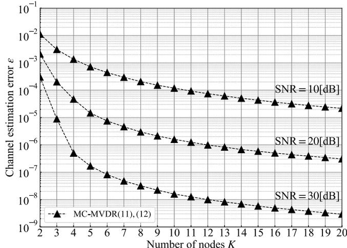
**Fig. 3.** Effect of the number of nodes and SNR on the channel estimation error.
