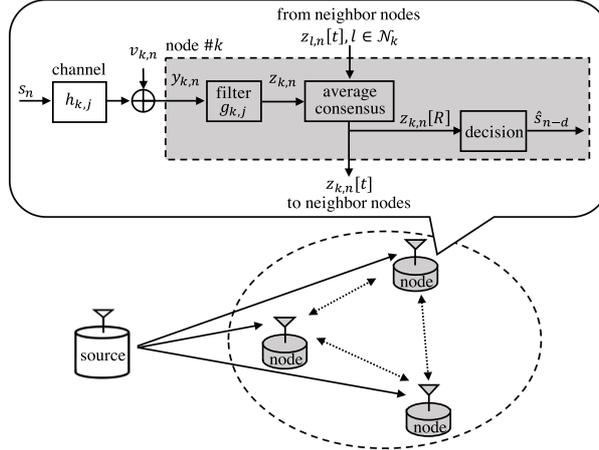
Fig. 1. System model of distributed equalization.
