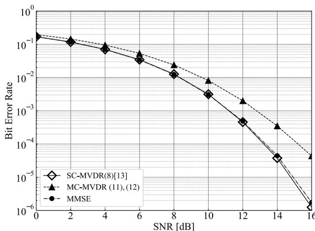
**Fig. 2.** BER performance comparison of centralized equalizers.
